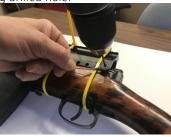
\*Ensure that the tap and drill angles are perpendicular (90°) to the mount at all times.
